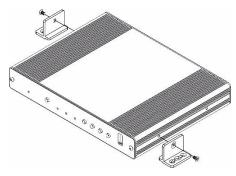
Mount the unit in a rack using the recommended rack adapter (see www.kramerav.com/product/KDS-SW2-EN7).
